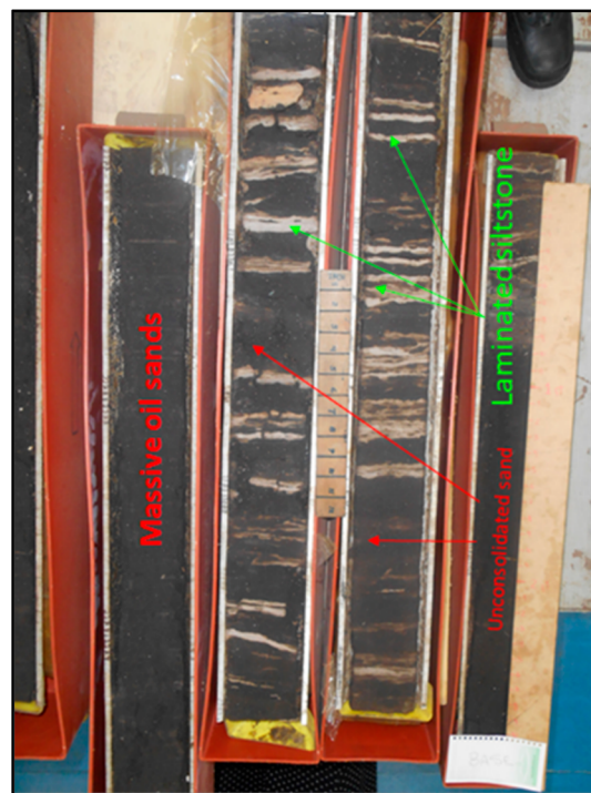
Figure 14. Reservoir samples from La FPO: massive unconsolidated oil sands with vertical heterogeneities. 81 Reprinted with permission from Rodriguez, 2016, 81 Copyright Université Sorbonne Paris Cité, 2016.
