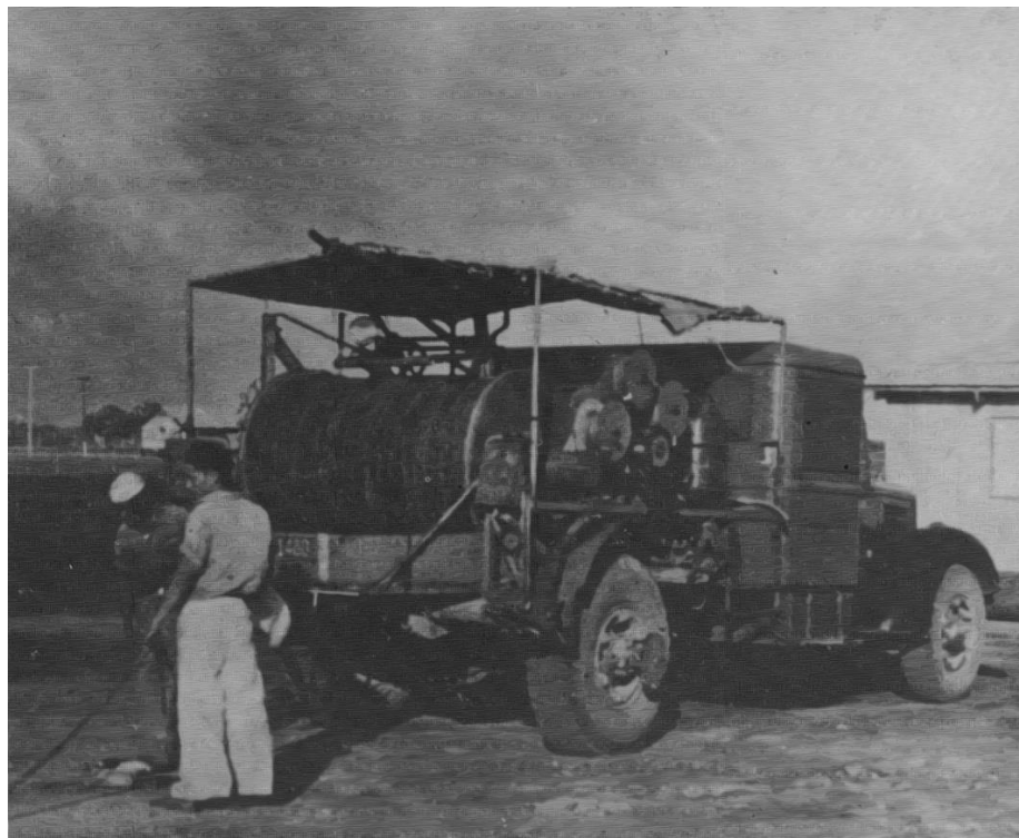
Figure 4. Old Schlumberger logging truck, used at that time in Venezuela. Source: Schlumberger
