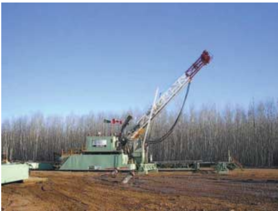
^ Angled drill rig in the shallow Mackay River field, operated by Petro-Canada ( right ). Wells dive at a 45° angle so they can make the turn to horizontal by the target depth of 400 ft [122 m] ( left ).
