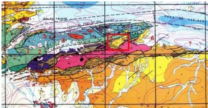
Fig. 1 Geologic and structural map of north-central Venezuela (after Bellizzia et al., 1976). Red box approximately corresponds to Fig. 2 and locates the River Tuy basin within the metamorphic nappes. Numbers label all basins from west to east: 1- Nirgua, 2- Miranda, 3- Bejuma, 4- Lake Valencia, 5- Tuy, 6- Barlovento and 7- Unare shelf
