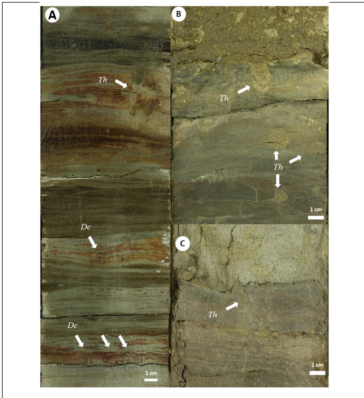
Figure 5.7 (A) Thalassinoides isp. (Th) in the Glossifungites Ichnofacies. Note presence of desiccation cracks (Dc) in the mudstone. H well, 566 m. (B) H well, 586 m and (C) Close up of Thalassinoides isp. Colonization took place after erosion exhumation and transgression.
