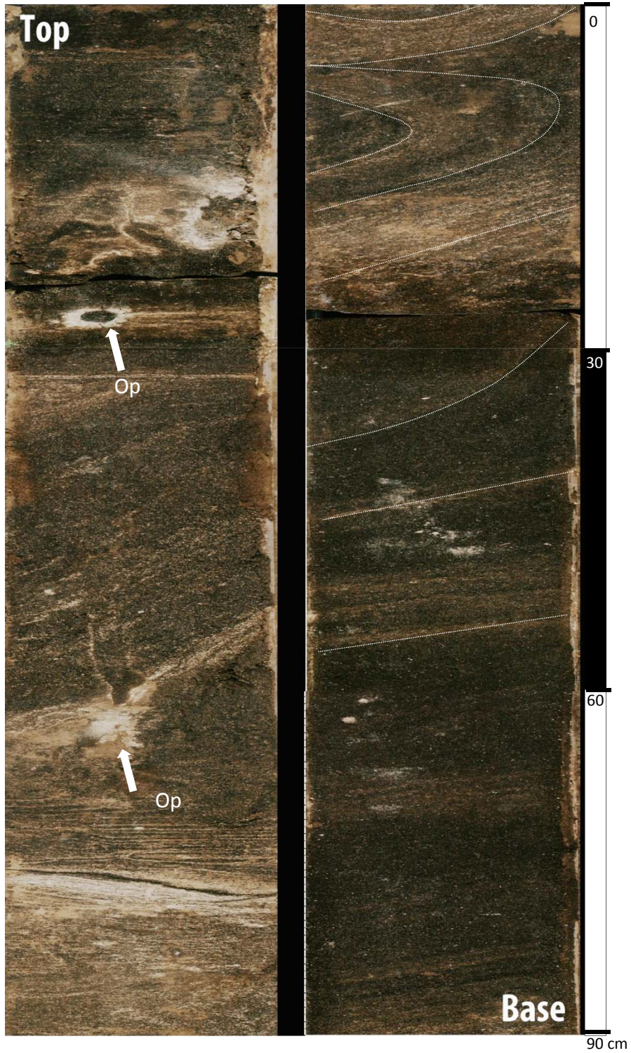
Figure 4.3 General view of FA2 with convolute lamination and Ophiomorpha nodosa in FE. B Well, 537.3-537.9 m.. Core width is 10 cm.
