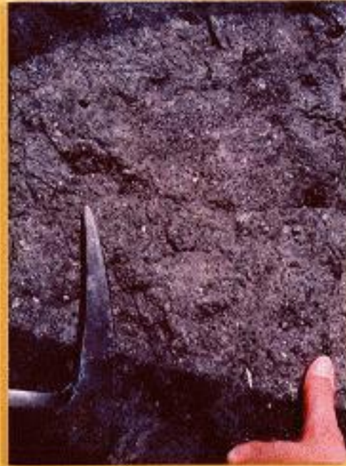
LOBATERA MINE, DETAIL OF PHOSPHATE ORE WITH FORAMINIFERA AND FISH REMAINS.
