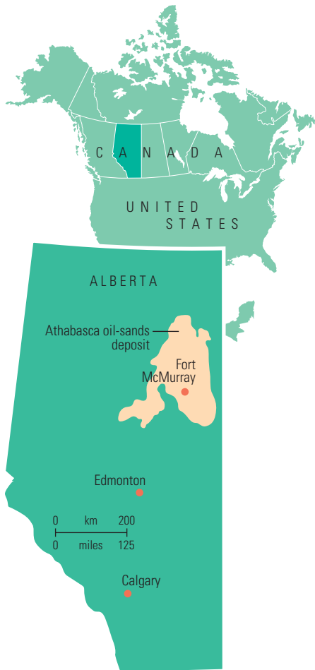
^ Athabasca oil-sands deposit. Alberta's oil sands, also called tar sands, contain more than 400 billion m 3 [2.5 trillion barrels] of bitumen in place, giving Canada the largest reserves of ultraheavy oil and bitumen in the world. The Athabasca deposit holds the vast majority of Canada's bitumen reserves.
