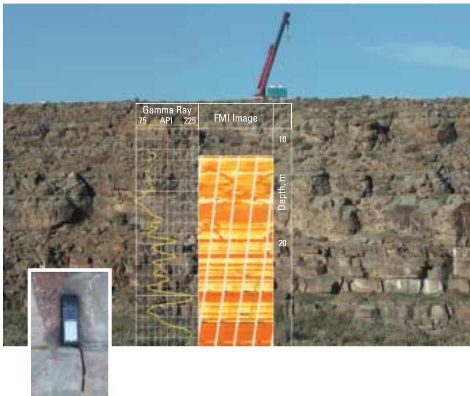
▲ Mapping the outcrops. High-quality outcrops, such as this one exposing Fan 4 below the NB2 well location, enabled the NOMAD team of geologists to map the sedimentological details of the fan complex. Accurate mapping was facilitated by global positioning systems (GPS) and geographic information systems (GIS) ( inset ). The FMI image and gamma ray log from the well immediately adjacent to the outcrop are overlaid and compare directly with the outcrop.
