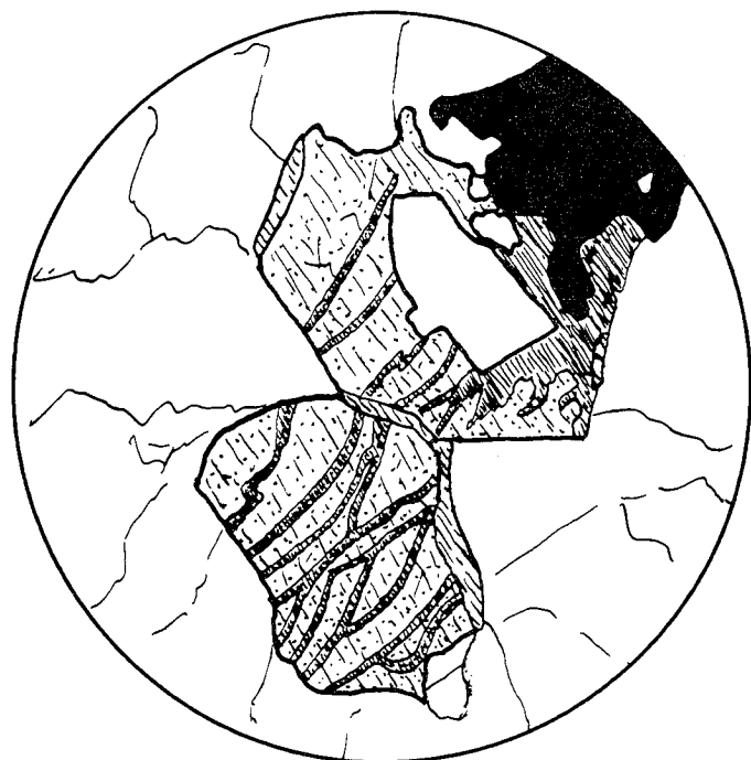
Fig. 5 Short and Steenken. Medium-grained charnockite. Quartz (white) enclosing hypersthene (dotted, showing cleavage). "Maschenstructure" with fine-grained biotite replacing hypersthene. Also amphibole (cleavage) and magnetite (black) are shown. 30 x (ordinary light), Sh 2002A.
