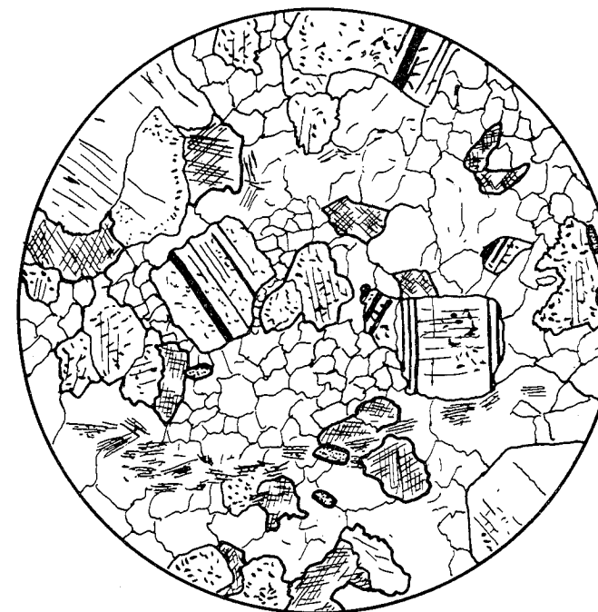
Fig. 13 Short and Steenken. Epidote-mica-microcline gneiss. Phenocrysts or porphyroblasts of poikilitic plagioclase and microcline in an uneven grained matrix of mainly quartz. Further shown are flakes of biotite and grains of epidote (dark outline, dotted). 10 x (crossed nicols), Sh 2180.
