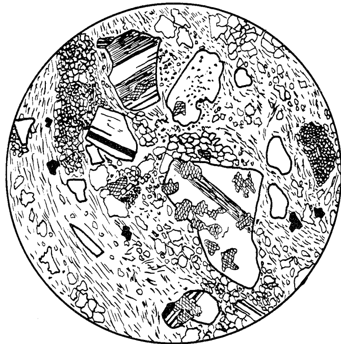
Fig. 9 Short and Steenken. Dacitic tuff consisting of (generally sharp edged) fragments of: quartz (white) plagioclase (albite twinning cleavage and enclosures of muscovite) as well as grains of groundmass in a very fine-grained matrix, partly made up of quartz and feldspar, partly of sericite (dashed), calcite (cross-hatched) and ore minerals (black). 35 x (crossed nicols). Sh 2274.
