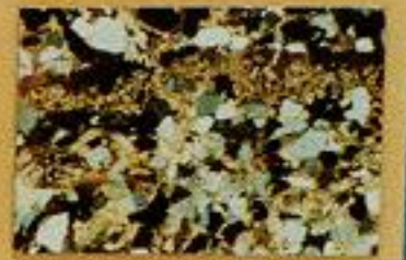
Transformation of fibrous illite into microcrystalline and sparse calcite within the structure of an equidistant sheet. X 1000x
