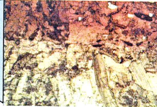
Molluscan packstone, strongly cemented by calcite and stylolitized
