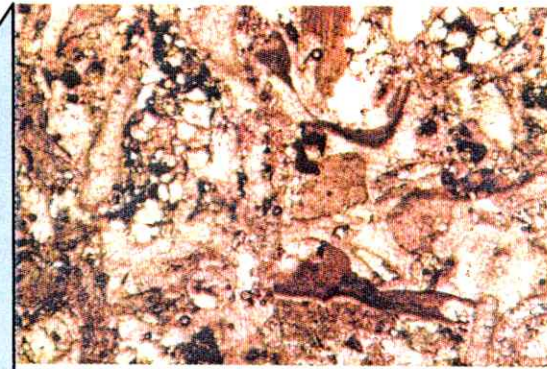
Equinoid-molluscan packstone, tightly cemented by calcite and dolomite
